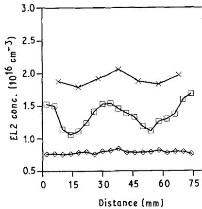
Figure 5 EL2 concentration profiles across the diameter of the wafers. For key, see Fig. 1.
