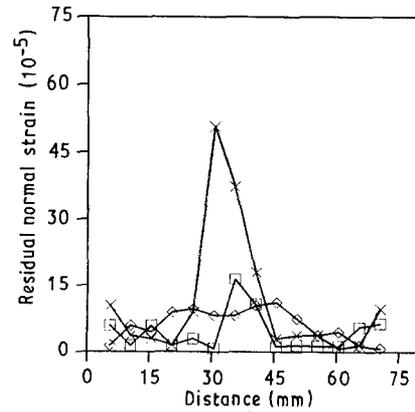
Figure 3 Variations of residual strains across the diameter of the wafers. For key, see Fig. 1.
