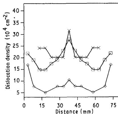
Figure 2 Dislocation density profiles across the diameter of the wafers. For key, see Fig. 1.
