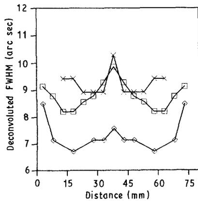
Figure 1 Variations of FWHM across the diameter of the wafers. (x) High gradient, undoped; (□) low gradient, undoped; (◇) low gradient, indium-doped.
