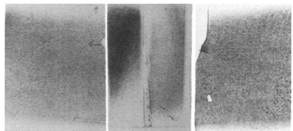
Figure 4 The X-ray Berg-Barrett topography of the undoped GaAs wafer grown under the high thermal gradient growth conditions ( $\text{CuK}\alpha_1$  radiation, (224) reflection, magnification 2x).
